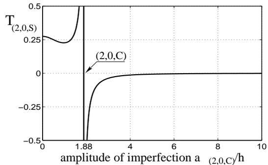
Figure 5. Type of non-linearity for mode (2,0,S) for an imperfection having the shape of mode (2,0,C).
