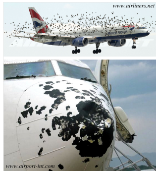
Bird impact traces on aircraft's nose
