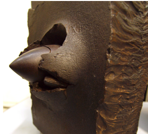
Sherman Firefly armor piercing shell on Tiger tank armor, Bovington Tank Museum Andy's photo www.flickr.com
