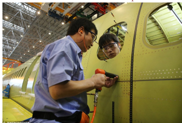
Fuselage of modern aircrafts contains \approx 100\,000 rivets
