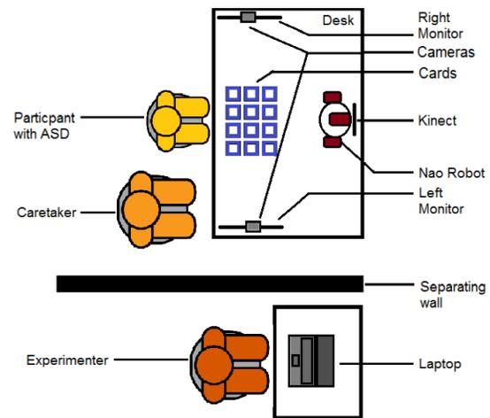
Figure 1 Setup of the Joint Attention task experiment
