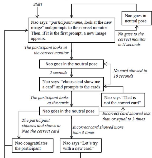
Figure 5 Diagram of the game stages with the robot Nao drawings (Figure 2), the ones in the second subset are more complex drawings (Figure 3), and the ones in the third subset are photos (Figure 4). Each subset is composed of five images: a tree, a bike, a car, a house, and a teddy bear. The cards are composed of the images printed on white paper on squares with sides 6 cm long, glued on a blue squared cardboard with sides 10 cm long.
