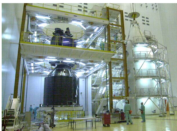
Picture 5.3.4.b – SYLDA 5 Internal carrying structure
