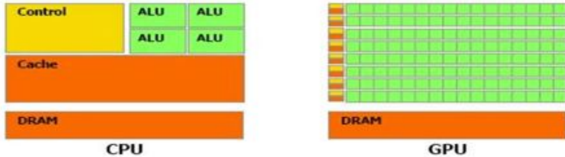
Fig. 3.3 Comparison between the architectures of the CPU and the GPU (courtesy of Kirk et al. 4) )
