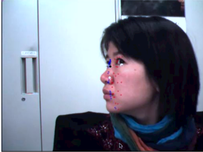
Fig. 5.3 Sparse template tracking can detect a large range of face orientation, contrarily to the haar face detection
