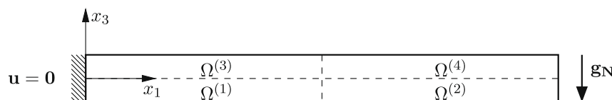
Fig. 1. Model of cantilever beam with four subdomains.
