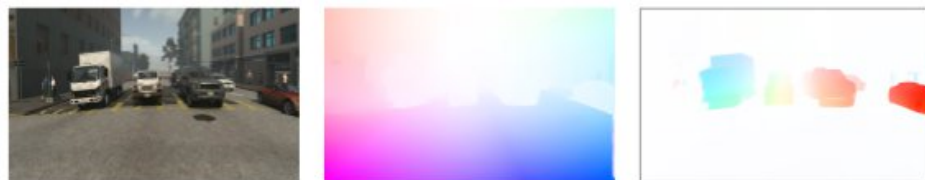
Illustration of the benefit of ego-motion compensation for scene recognition: optical flow map before (middle) and after compensation (right).
