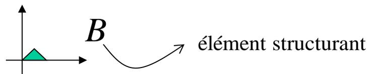
$$\varepsilon_B(X) = \overline{\delta_B(\overline{X})} = \overline{\overline{X} \oplus \check{B}} = \overline{\bigcup_{b \in \check{B}} \overline{X_b}} = \bigcap_{b \in \check{B}} X_b$$
