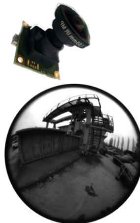
Semi-Dense SLAM with omnidirectional camera
