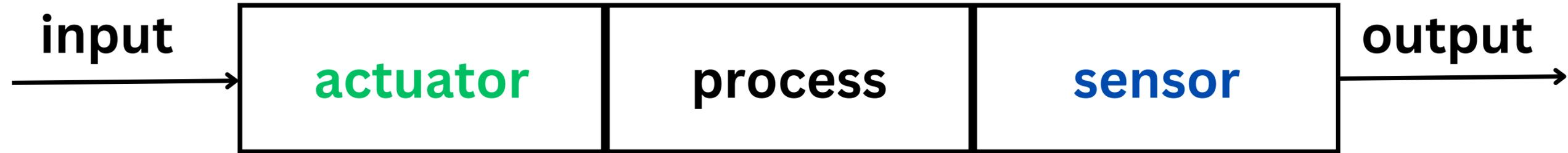
An **actuator** is a part of a device or machine that converts energy, often electrical, air, or hydraulic, into mechanical force. It is the component in any machine that enables movement.
