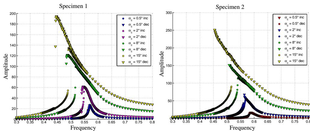
Figure 3: Frequency response curves of the two specimen. Inc. and Dec. refer to increasing and decreasing frequencies respectively.
