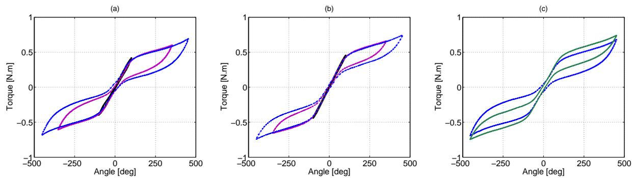
Figure 2: Quasi-static measurements at 0.01 Hz. Torque as function of the rotation angle, for three different imposed angle amplitudes (100, black, 350, purple and 450 degrees, blue). (a) specimen 1 ; (b) specimen 2; (c) comparison of the two specimens 1(blue) and 2(green) at 450 degrees.
