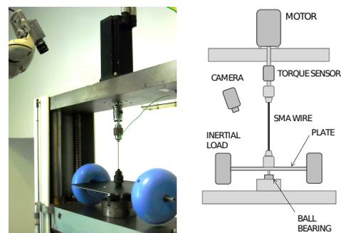
Figure 1: Photograph of the experimental setup (left) and schematic view showing the main components (right).
