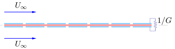
Figure 1: Schematic view of a plate in an homogeneous axial flow, equipped with small length piezoelectric patches on both sides. Each piezoelectric pair is shunted with a resistance like the one sketched on the left, modeling the electrical energy absorption.
