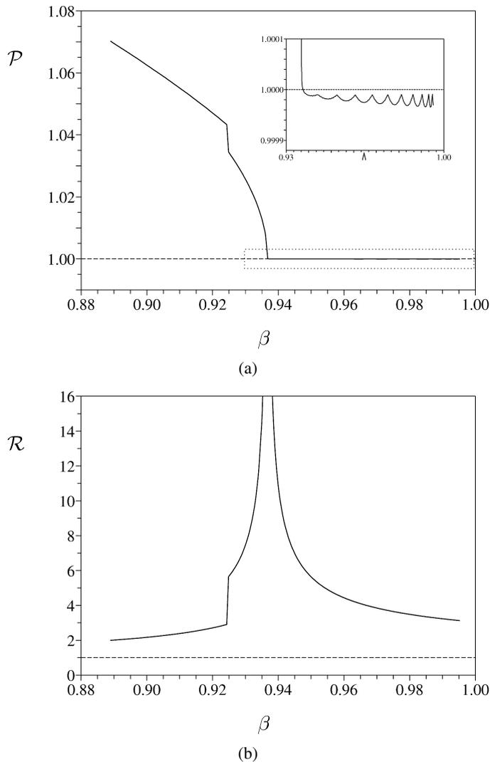
Fig. 5. (a) Value of  $\mathcal{P}$  above the instability threshold as function of  $\beta$  in the range of convective instability; (b) value of  $\mathcal{R}$ . The jump appearing for both  $\mathcal{P}$  and  $\mathcal{R}$  at  $\beta = 0.925$  corresponds to an abrupt change of  $l_c$ , see Fig. 1(b).
