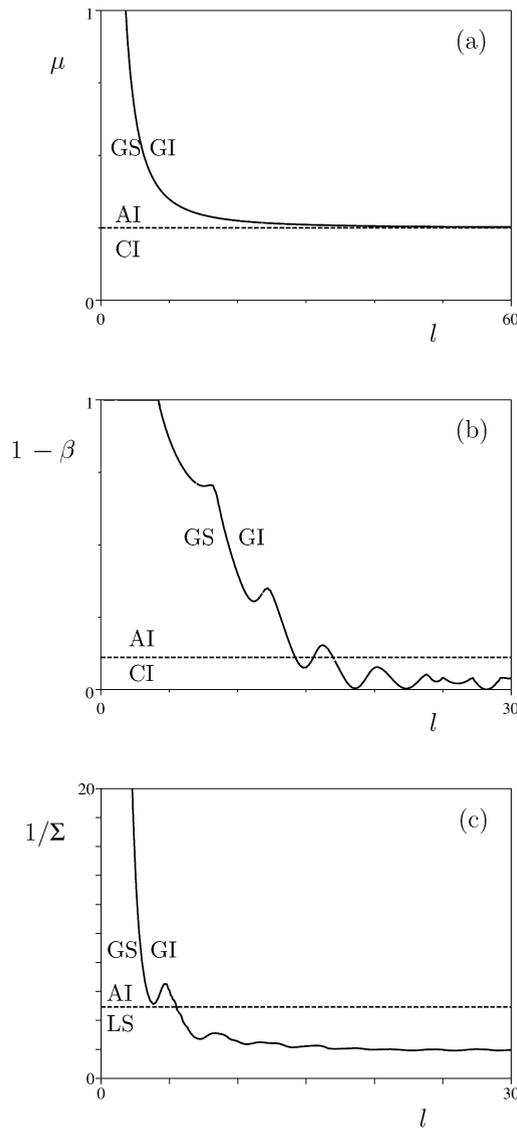
Fig. 1. Local versus global instability properties in the space of parameters; (GS), global stability; (GI), global instability; (AI), absolute instability; (CI), convective instability; (LS), local stability; (a) Ginzburg–Landau equation; (b) Bourrières equation; (c), Roth equation with  $\beta = 0.1$ .
