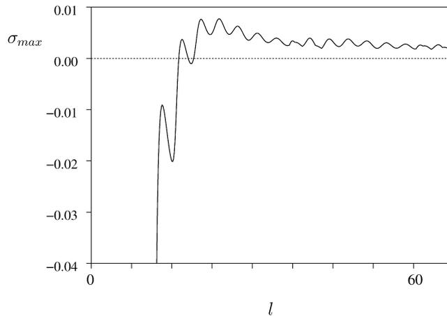
Fig. 6. Growth rate of the most unstable mode of a cantilevered fluid-conveying pipe on elastic foundation (Roth equation) as function of length for  $\beta = 0.2$  and  $\Sigma = 0.198$ ; (.....) maximum growth rate for  $l \rightarrow \infty$  predicted by the Kulikovskii criterion.
