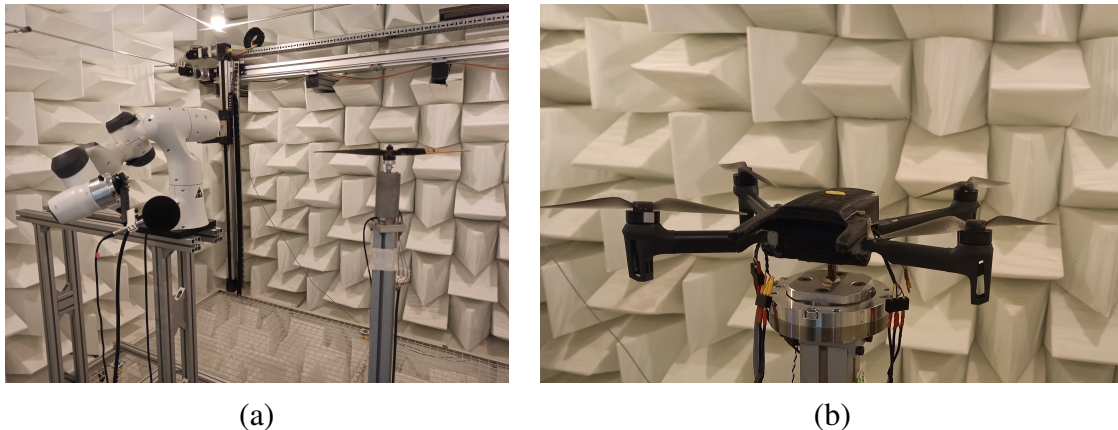
Figure 1: Experimental setups in the anechoic chamber of ENSTA Paris: (a) isolated propeller with robotic arm [1] and (b) quadcopter model mounted on a force balance.
