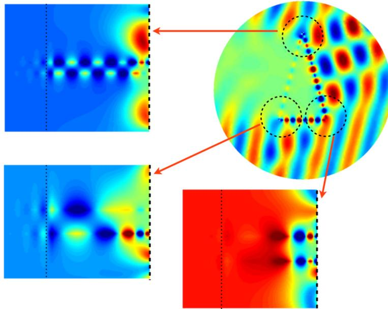
**Fig. 12.** Numerical solution in  $D_R$  with PMLs for  $\omega = 9$  PHz ( $\kappa_\varepsilon = -1.1838$ ). The bold dashed lines correspond to the interfaces where matching is made, the small dotted lines represent the boundary of the PMLs. Note that for the chosen incidence  $\alpha^{\text{inc}} = -\pi/12$  ( $330^\circ$ ), there is no trapped energy at the right corner (see also Fig. 13).
