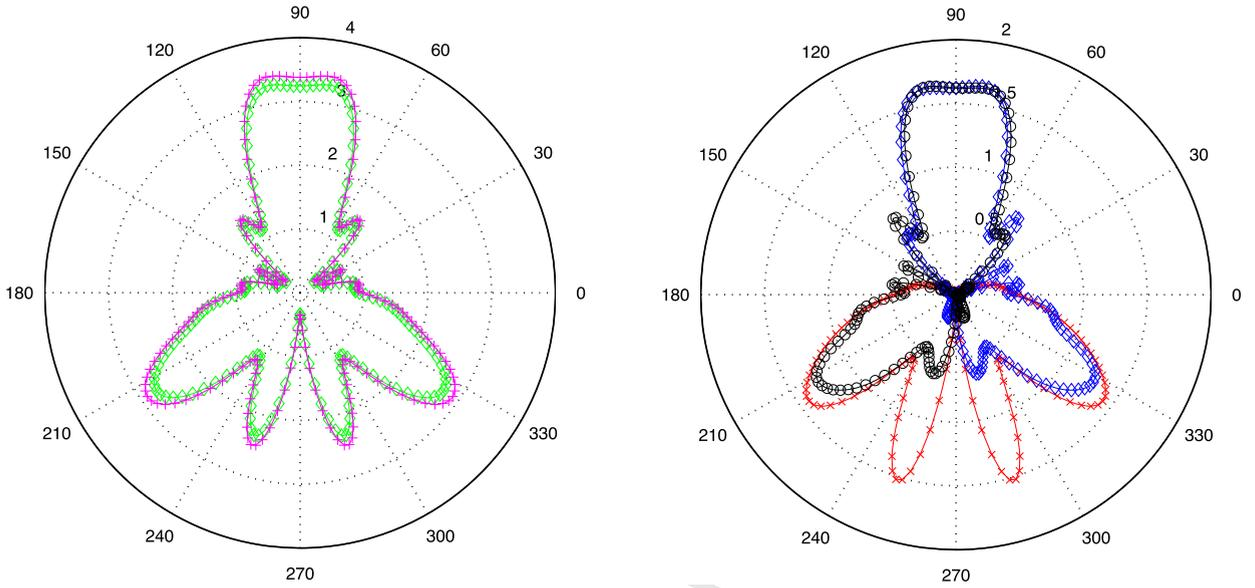
**Fig. 13.** Left: sum of the energy fluxes at the corners (diamond) and energy flux through  $\partial D_R$  (cross) with respect to  $\alpha^{\text{inc}} \in [0; 2\pi)$  in polar coordinates. Right: energy flux at the top corner (cross), left corner (diamond), right corner (circle) in polar coordinates. The frequency is set to  $\omega = 9$  PHZ ( $\kappa_\varepsilon = -1.1838$ ).
