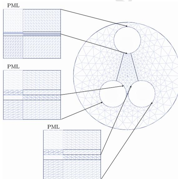
Fig. 10. Example of (very coarse) mesh. The arrows show the matching nodes between the different meshes.
