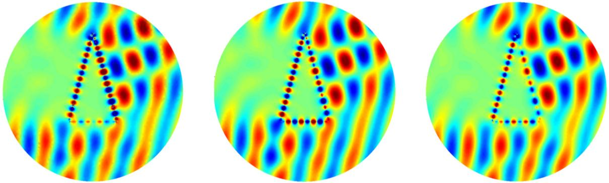
**Fig. 6.** Solution obtained using a standard P2 finite element method for different meshes: from left to right, 13273 nodes, 56031 nodes and 100501 nodes. The frequency is set to  $\omega = 9$  PHZ ( $\kappa_\varepsilon = -1.1838$ ). Note that the computed field is not stable at the interface when we refine the mesh.
