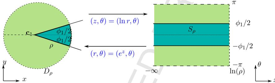
**Fig. 7.** Change of variables at the corner. The disk  $D_\rho$  is transformed into a semi-infinite strip  $S_\rho$  (the waveguide) with periodic conditions in  $\theta$ . As  $r \rightarrow 0$ ,  $z$  tends to  $-\infty$ .
