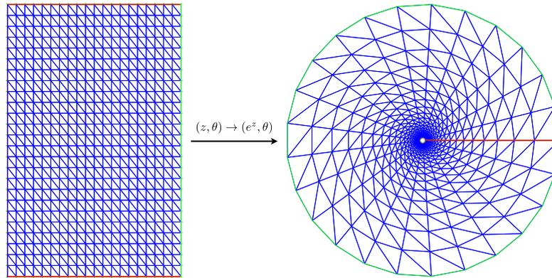
Fig. 9. Left: mesh of  $S_\rho^L$ . Right: obtained mesh with the change of variables  $(z, \theta) \mapsto (e^z, \theta)$ .
