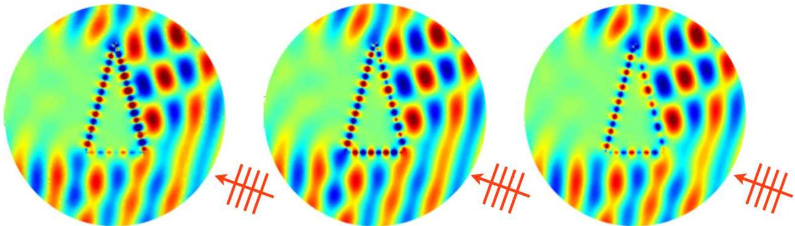
The numerical solution varies with the meshsize (especially near, or on, the interface).
