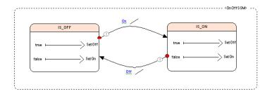
**Note:** the content, *i.e.*, the computations, of a state is defined graphically by dataflow diagrams or even other state-machines or both.
