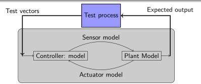
Simulation platform: Matlab/Simulink/Stateflow
