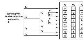
a, b, c, d, e, f, g, h represent the necessary minimum risk reduction. The link between the necessary minimum risk reduction and the safety integrity level is shown in the table.
