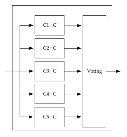
N-Modular redundancy where
