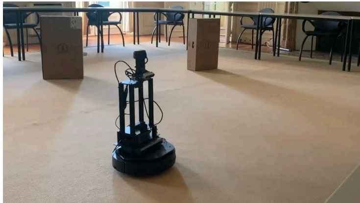
Figure: A Locobot robot at Naver Labs Europe navigating in a real environment, learning to avoid obstacles [SBC+2022].
