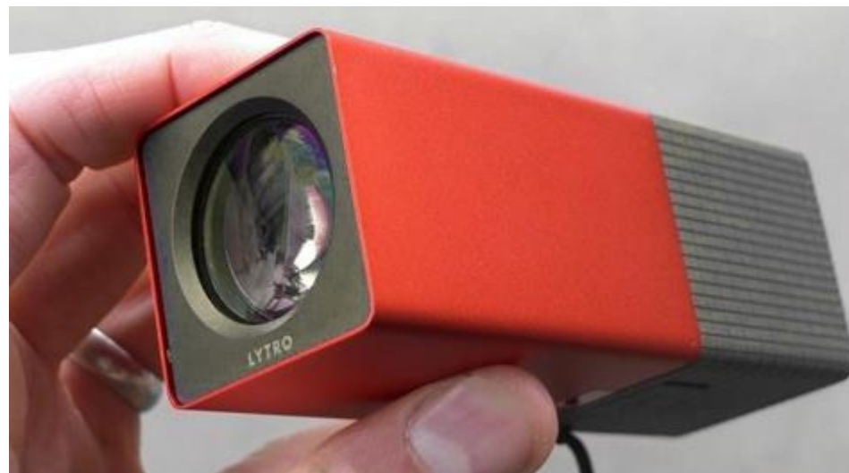
Light field plenoptic camera Lytro™
