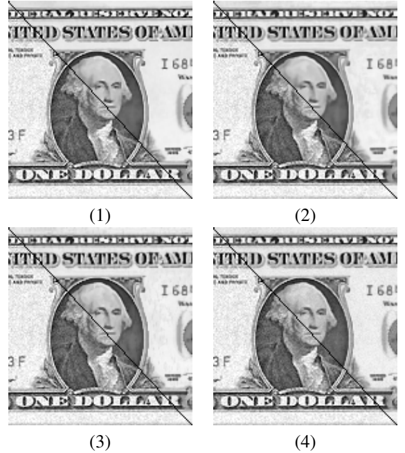
Figure 6. NL-means filtering in the local jet feature space. (1) LR ( \mathcal{N}(\mathbf{x}) : 17 \times 17 neighbourhood of \mathbf{x} in the image domain). (2) UR, exact search ( \mathcal{W}(\hat{\mathbf{x}}_f) : 30 NN in the local jet domain), (3) UR, approximate search ( \epsilon = 10.0 ), (4) UR, approx. search, with quantised feature space (1938 words in the dictionary).
