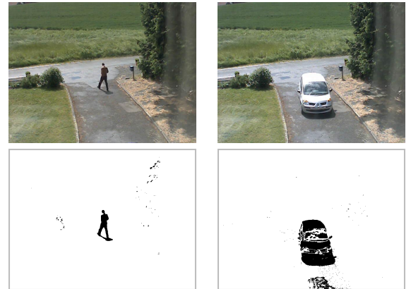
Figure 10. Background subtraction based on sample and consensus using a codebook of colour local jet features.
