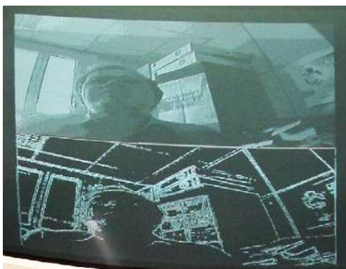
Figure 7: The results on a VGA monitor: the camera stream (above), the contours (below).
