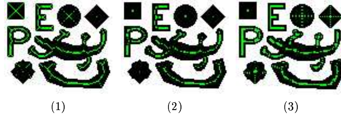
Fig. 3. (1) S_4(X) the morphological skeleton based on d_4 . (2) S_{(4,8)}(X) the mixed median axis. (3) S_8(X) the morphological skeleton based on d_8 .
