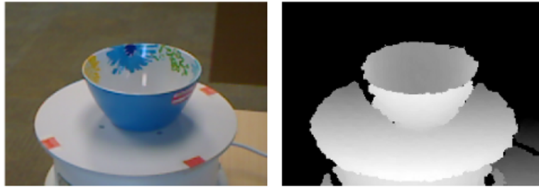
Figure 1.5: Example of RGB-D data, taken from[Lai+11]. For depth (right), bright colors indicate lower depth (and thus closer object to the camera plane)
