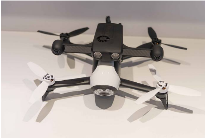
Figure 1.6: Example of a stereo camera placed on a UAV in order to compute a depth map (here, a Parrot Slam Dunk on top of a Bebop2)
