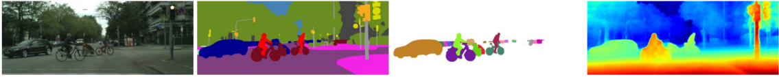
Figure 7.1: Multiple different but correlated semantic levels of a particular scene. From left to right: input, semantic segmentation masks, instance masks, depth. Figure taken from Kendall et al. [KGC18]
