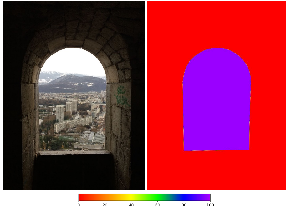
Figure 6.2: Example of a multi-modal depth distribution scene with corresponding depth: foreground is much closer than mean depth and background further.
