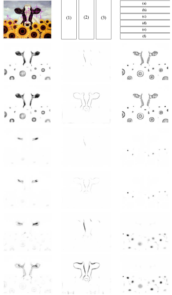
Figure 3. Similarity maps based on 2-order local jet metrics, for 3 different pixels: (1), (2) and (3), and 6 different distances: Single (same) scale: (a) canonical components (CC), (b) rotation invariant components (RIC), Pan-scalic (4 scales): (c) CC, (d) RIC, and Trans-scalic (4 scales): (e) CC, (f) RIC. For each pixel \mathbf{x}_0 , the similarity map is defined as M_{\mathbf{x}_0}^{d_F}(\mathbf{x}) = \Phi(d_F(\hat{\mathbf{x}}_0, \hat{\mathbf{x}})) , with d_F the local jet distance, and \Phi(z) = 1 - e^{-\frac{z^2}{C^2}} , with C = 10 . (Painting by Lowell Herrero)
