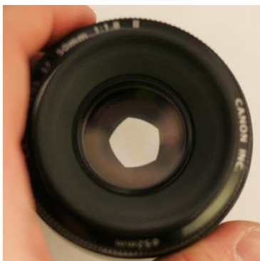
Traditional 5-blade diaphragm and the family \{g_d\}_{d \in D} of kernels.
