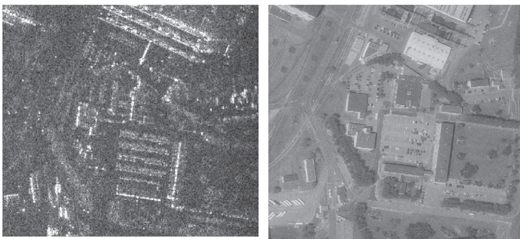
Fig. 1. Examples of the building appearance in the slant range SAR image with sensor viewing from the left (left) and the corresponding optical image (right).
