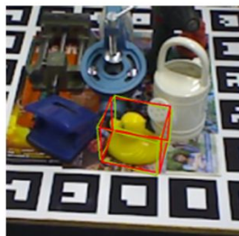
Figure 3. Visualization of predicted confidence score and ground truth 3D-IoU score. The green 3D bounding box depicts the box transformed with the ground truth pose, while the red box is transformed with the predicted pose. Below the images the individual predicted scores and ground truth scores are shown.
