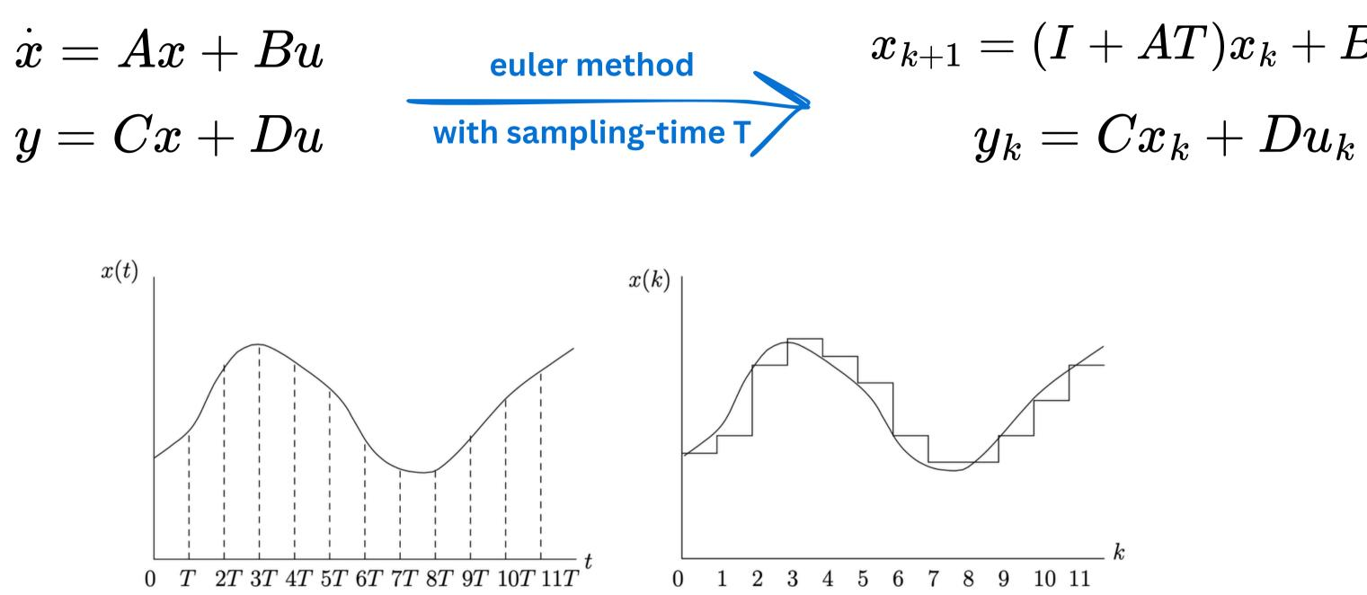
or they are obtained as a result of sampling (discretization) of continuous-time systems.
