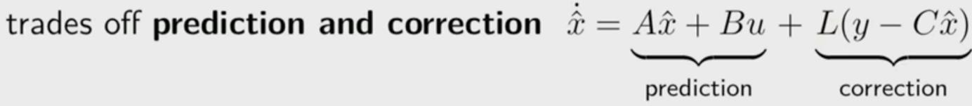
$\Rightarrow R \succ 0$  quantifies correction through measurement: R "large"  $\implies L$  "small"  $\implies$  trust prediction R "small"  $\implies L$  "large"  $\implies$  trust measurement
