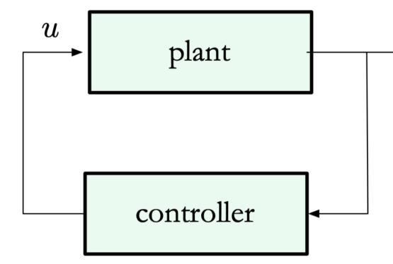
Full state feedback u = -Kx is *not implementable*!! In that case, an observer is used to estimate the state x:
