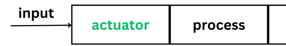
An actuator is a part of a device or machine that convert energy, often electrical, air, or hydraulic, into mechanical force. It is the component in any machine that enables movement.
